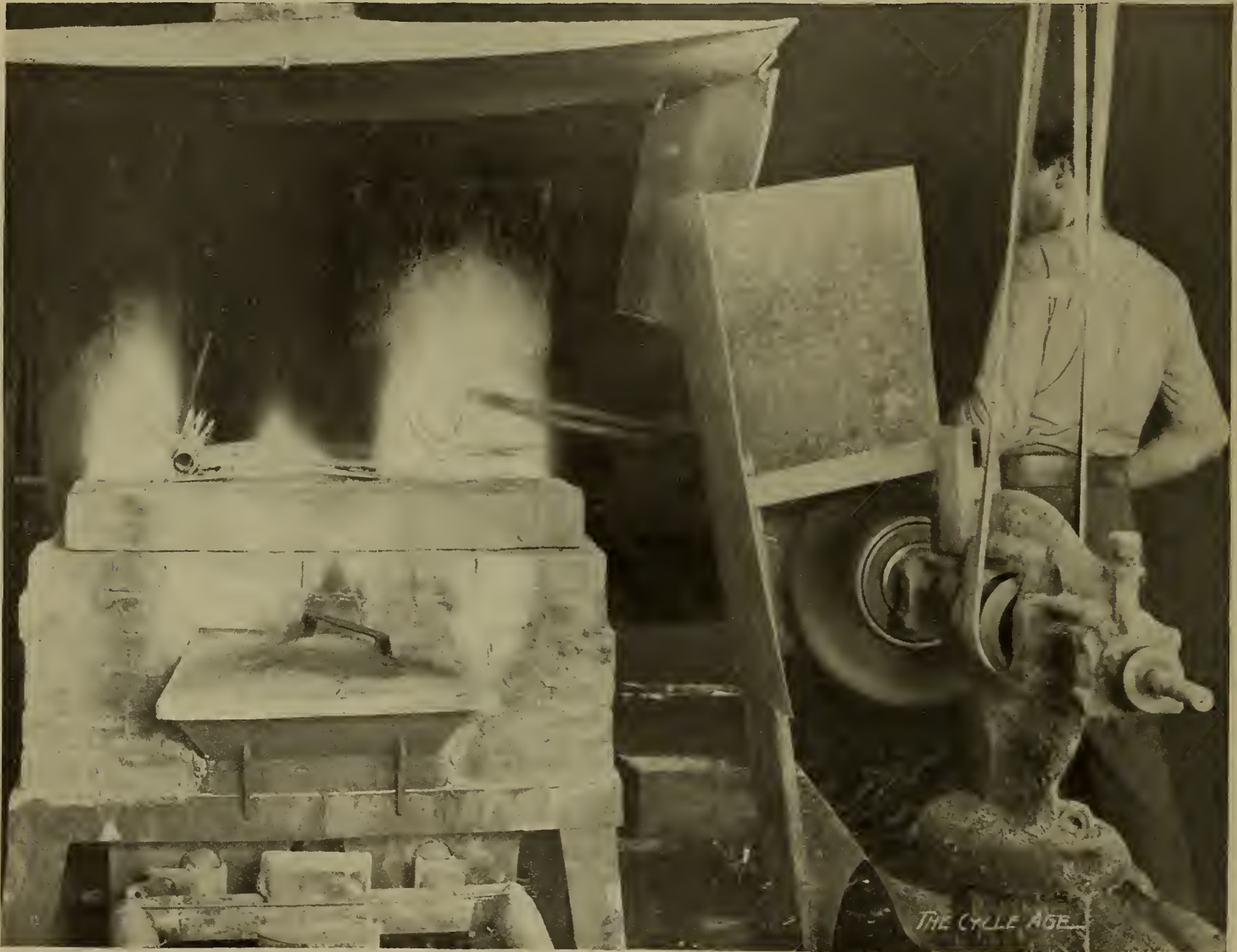
"CHICAGO" BRAZING FURNACE IN OPERATION—BRUSH WHEEL FOR REMOVING SUPERFLUOUS SVELTER AT THE RIGHT.
